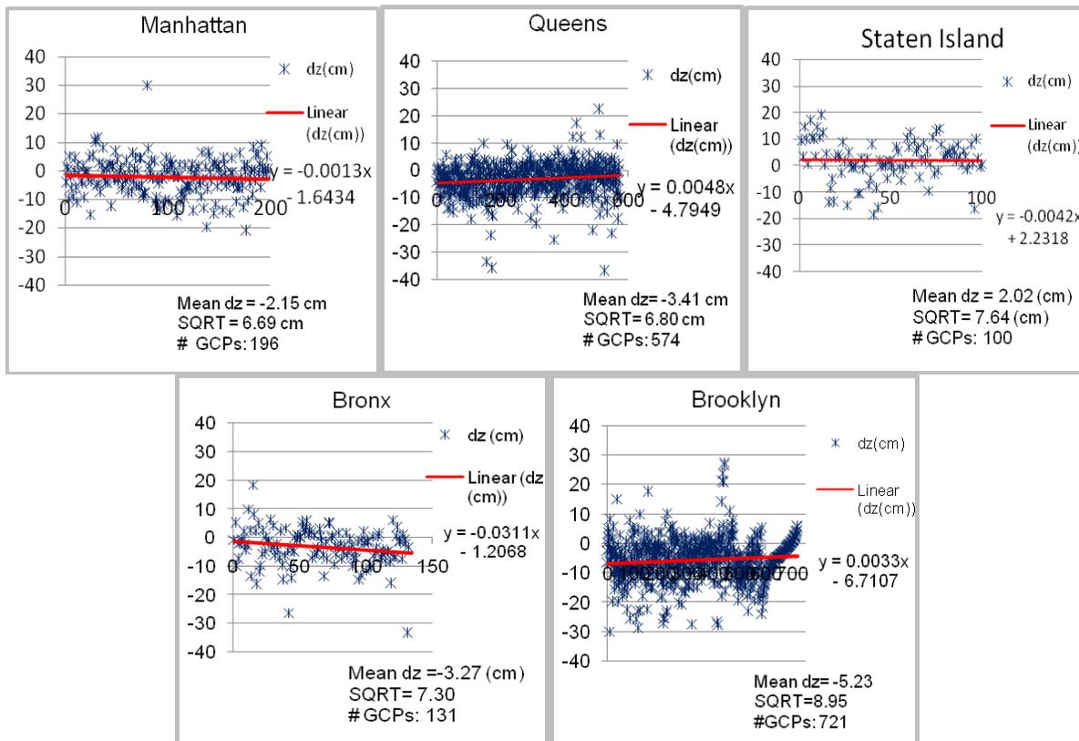
**Figure 2. Scatter diagrams of the mean of  $\Delta z$  between the ground checkpoints and the LiDAR z values for each borough in NYC.**
