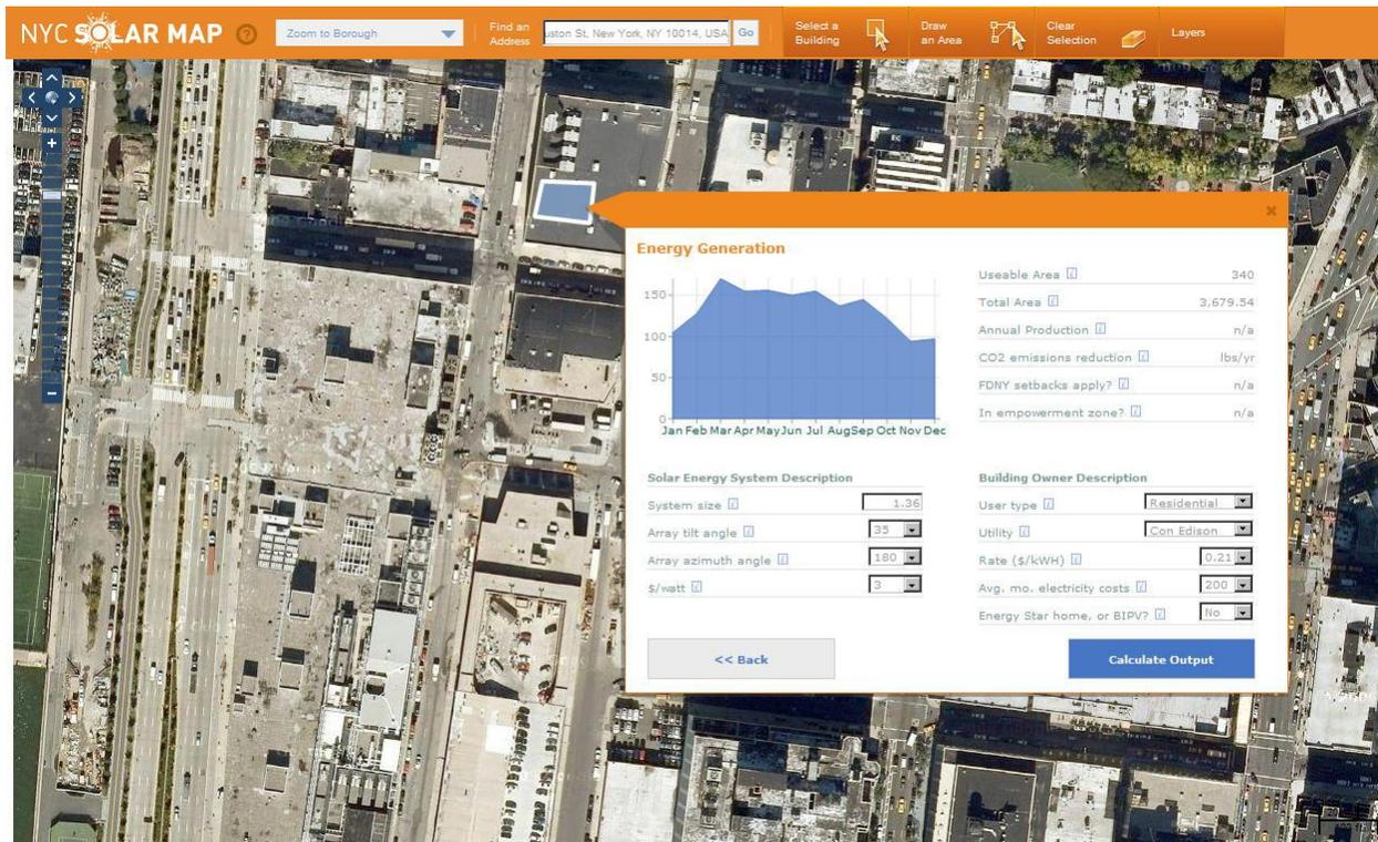
Figure 9. NYC SOLAR MAP showing energy profile for a user-generated polygon on a selected building
