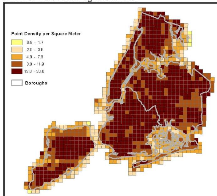
**Figure 3. LiDAR point density per square meter in NYC.**
