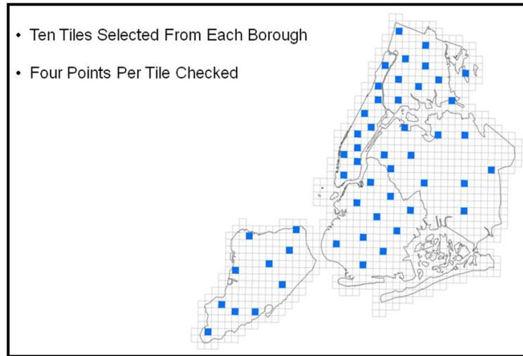
**Figure 4. The selected LiDAR tiles for horizontal accuracy assessment in .**
